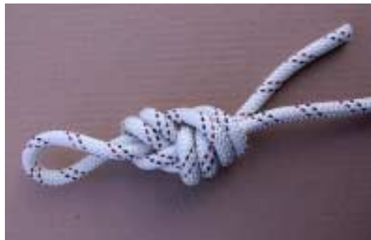
Figure 5 Double figure-of-ten knot
