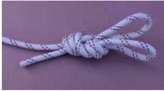
Figure 6 Double figure-of-eight on a bight
